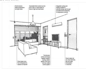
Fig: 3. General layout of Room with Light, Fan and Curtain
