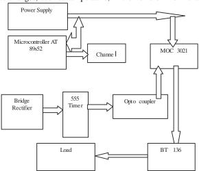
Fig: 1. Block diagram of light, Fan and curtain control
